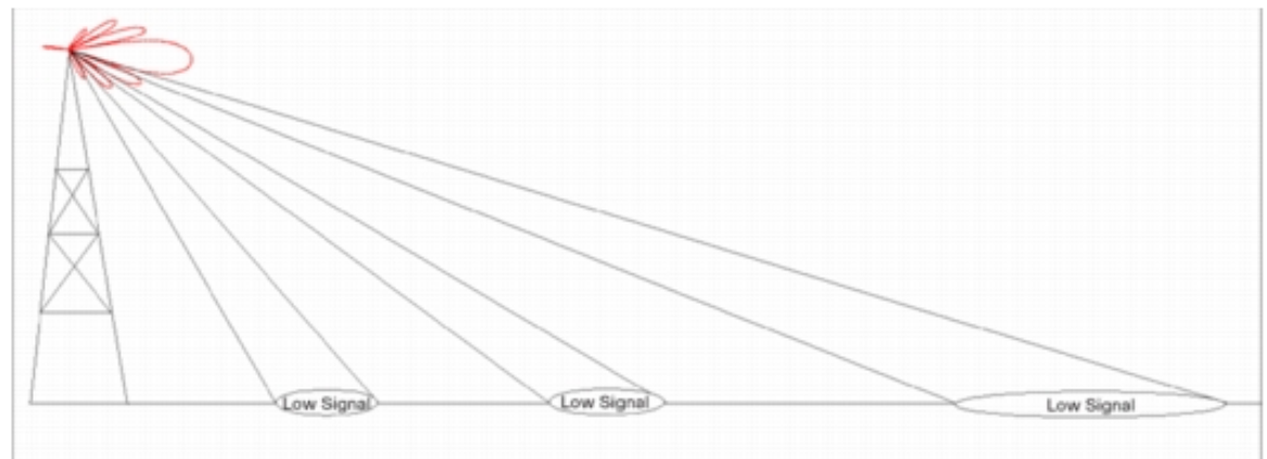
Coverage Gaps from Elevation Plane Nulls
