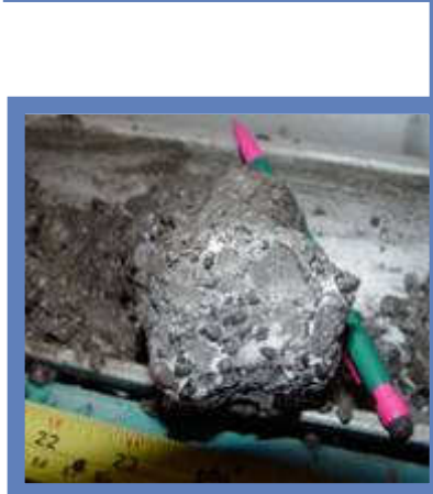
A large gas hydrate plug formed in a subsea hydrocarbon pipeline. Picture from Petrobras (Brazil)
