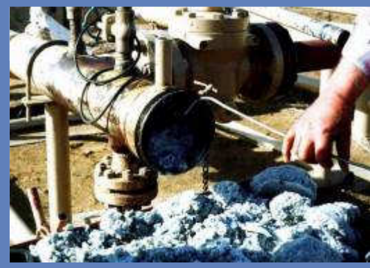
A large gas hydrate plug formed in a subsea hydrocarbon pipeline. Picture from Petrobras (Brazil)
