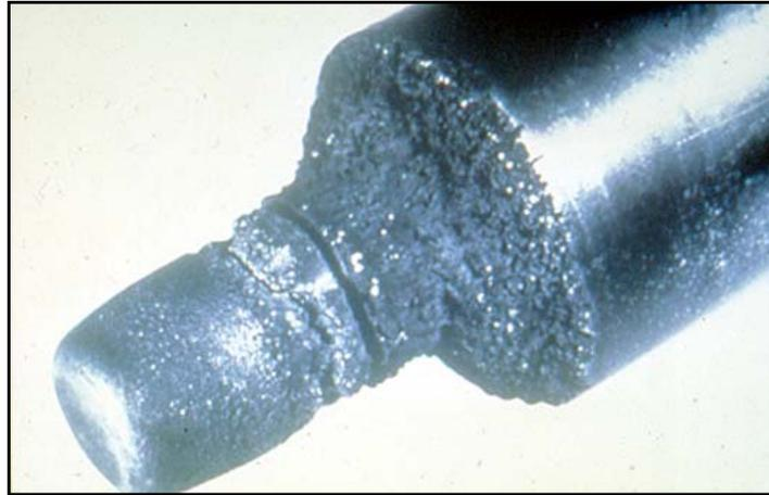
Figure 23-5. Actual Cavitation Damage of a Valve Plug
