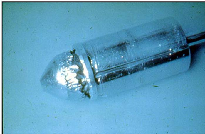
Figure 23-7. Actual Flashing Damage of a Valve Plug
